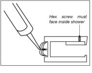
**4.** Ensure the glass receiver channel is located firmly over the base glazing channel. The machine recess in the wall glazing channel must firmly locate over the base glazing channel.
