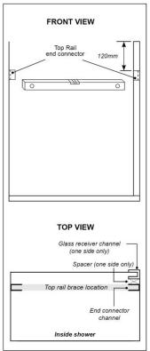
9. TOP RAIL BRACE INSTALLATION It is recommended that the top rail brace is fitted prior to tiling. AVOID SCRATCHING.
