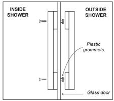
**11. ROLLER SET ASSEMBLY TO GLASS DOOR** Ensure the direction of the door is correct. Fit the plastic grommet through the glass first (note direction of grommet). Tighten with the 4mm Hex Key supplied.
