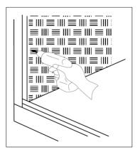
**6.** Apply a continuous bead of silicon to the full length of the channel and waterproofing, indicated by the dark line (inside channel).
