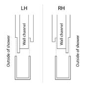
Locate the framing timber. Use the 4mm drill bit to drill holes through the glass receiver channel. Fix four screws through the channel in the wall framing (use wall plugs if required).
