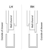
5. Locate the framing timber. Use the 4mm drill bit to drill holes through the glass receiver channel. Fix four screws through the
