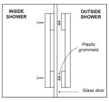
Assemble handles as shown. Use the 3mm Hex Key supplied with handle set.
