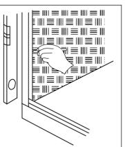
**3.** Apply a silicon seal to full length of channel. Silicon used must be compatible with anodised aluminium as well as the waterproofing being used.
