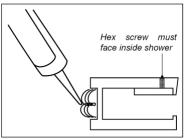
4. Ensure the glass receiver channel is located firmly over the base glazing channel. The machine recess in the wall glazing channel must firmly locate over the base glazing channel.
