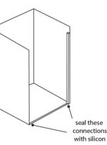
Prior to installation of glass panels and infill. All connections of channels, must be sealed with clear silicon supplied
