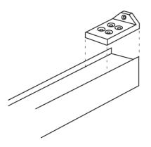
16. Stand inside the shower and manouver the preassembled door and top track inside the shower. Carefully lift the top track with the door attached into place over the return panel 20 MGF. The top track will sit on the wall channel on one side. Ensure the top track is level. Fix both MG-3W end connector brackets to the wall.
