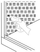
Apply a continuous bead of silicon to the full length of the channels and waterproofing, indicated by the dark line (inside channel).
