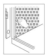
where the wall channel is plumb.  Apply a silicon seal to full length of the channel. Silicon used must be compatible with anodised aluminium, as well as acrylic or the waterproofing being used.
