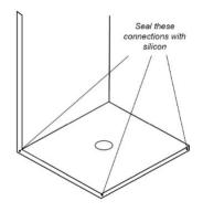
Prior to installation of glass panels and infill use the clear silicon supplied
