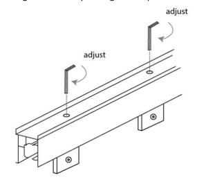
the top of the door hangers. Turn the key anticlockwise to lift the door.
