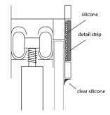
26. Clear silicone should be used to seal the end
