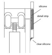
track. This will cover the adjustment holes. Do not silicone into place.
