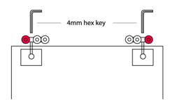
**14.** When the idle rollers are being fitted to hangers apply a 5mm drop of clear silicone inside the thread. This will ensure that the hanger does not move out of adjustment.
