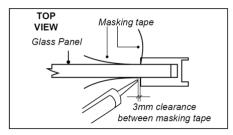
remove the excess silicon. Remove the masking tape immediately after application.
