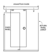
attached into place over the return panel **20 MGF.** The top track will sit on the wall channel on the fixed panel side and the MG-2W end connector angle will slide over the glass return panel. Ensure the top track is level. Fix the MG-3W end connector bracket to the wall. Tighten the screws into the end connector angle firmly.
