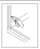
6. Apply a 10mm continuous bead of Flexicone, to the full length of each wall channel. Silicon seal the join where the wall and base channel will intersect. Screw the wall channels to the wall (ensuring they are plumb).
