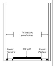
shown. Sill infill must measure 3mm larger than door, trim if required.
