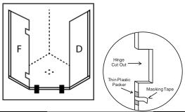
Hinge Installation. Atlantis glass (EXCLUDING 1930MM HIGH GLASS) is now coated with CristalCote glass protection in the factory. This coating may cause the hinge to slip after installation if not tightened enough. Atlantis recommends cleaning around the hinge cut out prior to fitting hinges. Clean both sides of the glass 15mm around the edge of the cut out with Fuelite (Fuelite is available from petrol stations).
