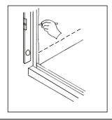
**3.** Ensure the glass receiver channels are located firmly over the base glazing channels.
