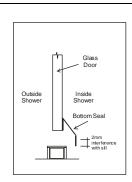
**25. Door Seal Installation** – install seals as shown. Trim the **Y SEAL** to length to fit between the hinges.
