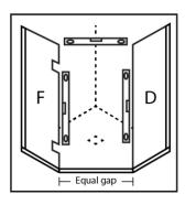
14. Fixing of glass panels into wall channels
