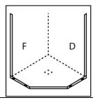
**11. Critical Seal.** Remove any dust and dirt first. Seal the connection between the glass receiver channel and the base glazing channel with clear silicon, prior to final glass placement. Ensure junction between wall channel and base channel is full of silicon before final glass placement.
