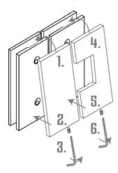
Fit the hinges. The removable cover (and bolts) must be on the outside of the shower. The reverse C holds the door and the other side goes onto the fixed panel
