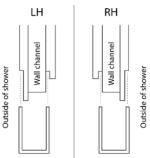
**4.** Apply a silicon seal to full length of channel. Silicon used must be compatible with anodised aluminium as well as the waterproofing used.
