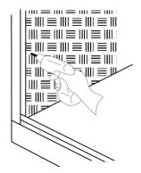
**6.** Apply a continuous bead of silicon to the full length of the channel and waterproofing, indicated by the dark line (inside channel).
