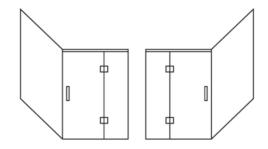
2. Position the glass receiver channels over the base glazing channels. Mark the wall to indicate where the wall channels are plumb.
