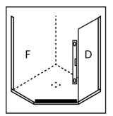
**13.** Locate panel **F** into channels and slide firmly to sill infill. Adjust this panel ensuring it is level and plumb to panel **D** by adding or removing packers in bottom channels.
