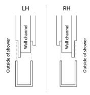
5. Locate the framing timber. Use the 4mm drill bit to drill holes through the glass receiver channels. Fix four screws through the channels into the wall framing (use wall plugs if required).
