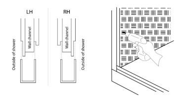
5. Apply a  $\parallel \equiv$ continuous bead તા≣∥ of white silicon to the full length of ≣₩≡₩≡₩≡ the channels and **₩**≣**||| || || ||** waterproofing membrane, indicated by the dark line (inside channels).
