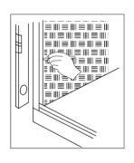
3. Apply a silicon seal to full length of channel. Silicon used must be compatible
