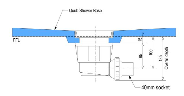
Ensure a minimum recess size of 250mm wide x 250mm long x 150mm deep for the channel drain and waste outlet
