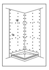
**Tiled Walls—** Wall Channels must be fitted onto waterproofing PRIOR TO TILING. See Screen Fitting Instructions
