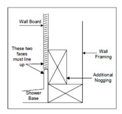
5. Place the base in finished positon. Leave the Protective film over it and the protective tape around the perimeter of the base.
