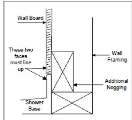
5. Place the base in finished position. Leave the Protective film over it and the protective tape around the perimeter of the base.
