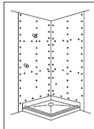
**Tiled Walls**– Wall Channels must be fitted onto waterproofing PRIOR TO TILING. See Screen Fitting Instructions
