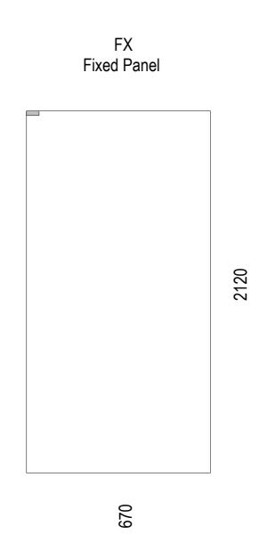
Supplied with glazing channels and top brace to fix glass to wall
