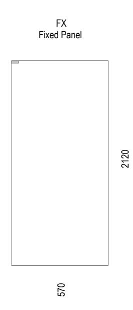
Supplied with glazing channels and top brace to fix glass to wall
