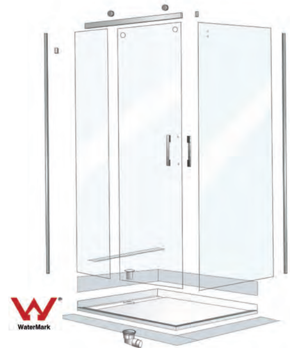
Illustration of 2-walled shower showing sliding door.
