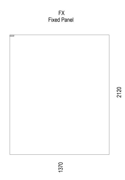
Supplied with glazing channels and top brace to fix glass to wall
