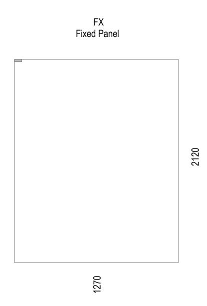
Supplied with glazing channels and top brace to fix glass to wall
