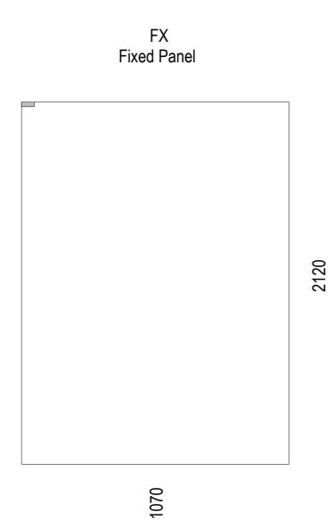
Supplied with glazing channels and top brace to fix glass to wall
